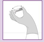
Close the lid of the incubation vial and shake vigorously by hand. Make sure that the extracted sample comes into contact with lid.
