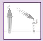
Remove the small cap to open the dropper tip. Transfer the extract to a fresh incubation vial.
