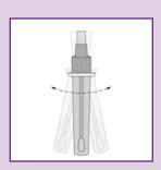
Place the swab into the tube, breaking it off at the pre-scored point. Close and shake for 1 min.
