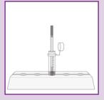
Add a test strip to the incubation vial and wait for 5 min. Ready! You can read the result.
